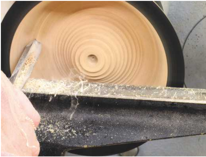
▲ Pic.1 To make the scraper more versatile and easier to use, it's worth grinding the tool with a downwards angle on the top; this creates the negative angle, or rake as it's known
